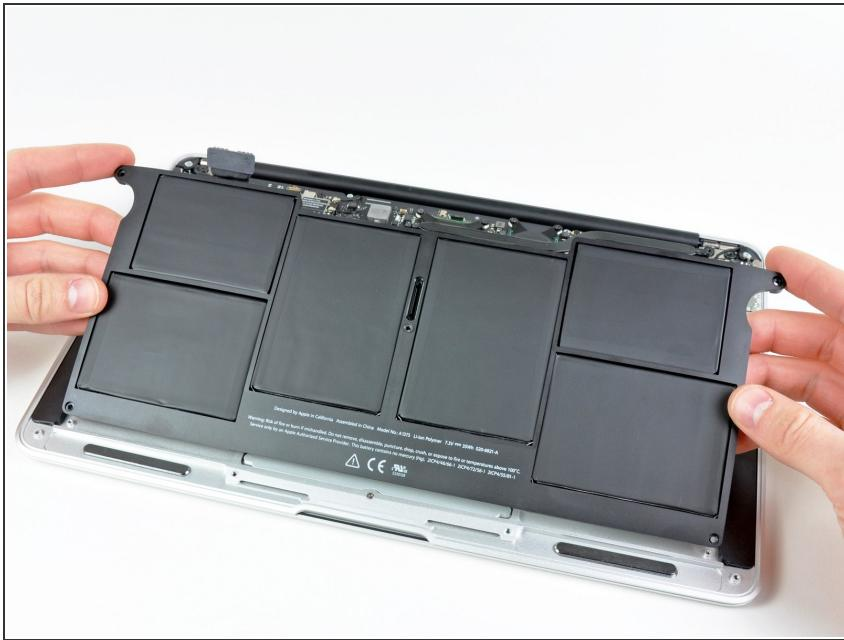
**⚠** Do not touch or squeeze the six lithium polymer cells when handling the battery.
